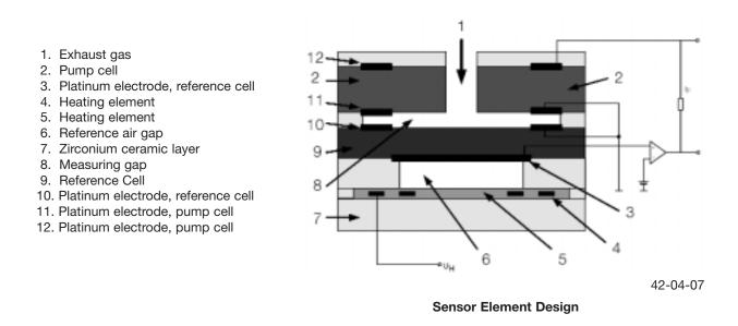
The pump cell (2) and reference cell (9) are made of zirconium dioxide and each coated with two porous platinum electrodes. They are arranged so that there is a measuring gap (8) of approx. 10 to 50 microns between them. This measuring gap is connected by an inlet opening to the exhaust gas (1). The pump cell is controlled by the ECM applying voltage to the electrodes to initiate oxygen ion pumping across the porous membrane of the reference cell, providing a quicker response time.
